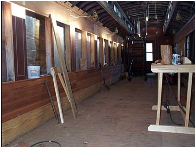
View down the length of the car showing the all new "bad" side and the original "good" side.
